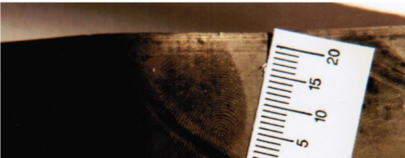
Metallic light fixture recovered from test fire scene. Item was completely covered in soot and located above point of origin. Fingerprints shown became etched into the metal, making them permanent.
